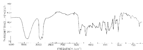
Fig. 3. Infrared spectrum of 5 \beta -cholestane-3 \alpha ,7 \alpha ,12 \alpha ,25-tetrol (VI, KBr disc).
